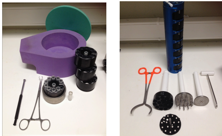
Figure 6 – Tools for cryocooling protein crystals
